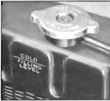
Figure 1-6—Radiator Filling Level—Cold
