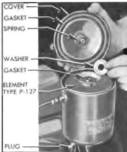
Figure 1-11—Changing Oil Filter Element
