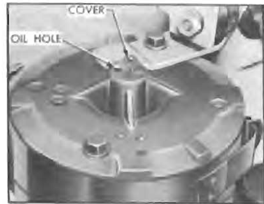
Figure 1-13—Power Unit Motor Oil Hole
