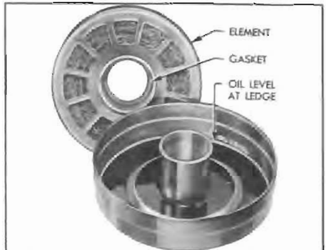
Figure 1-10—Air Cleaner Element and Sump
