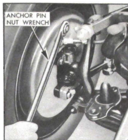
Figure 8-9—Using Anchor Pin Nut Wrench J 854
