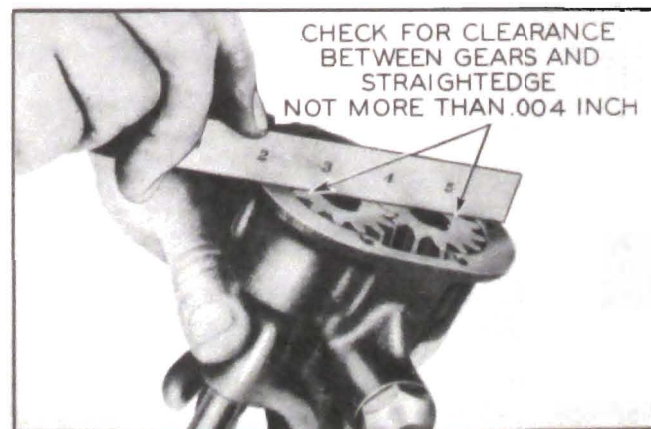
Figure 2-38—Checking Clearance of Gears at Cover
