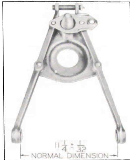
Figure 6-22—Correct Spacing of Control Arm Inner Ends
