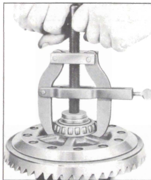
Figure 5-11—Removing Differential Bearing Using Puller J 2241
