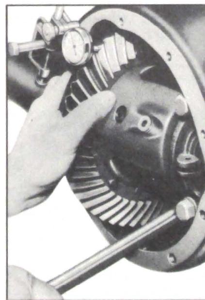
Figure 5-31—Checking Backlash with Dial Indicator
