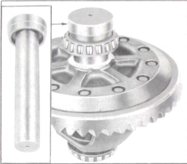
Figure 5-12—Installing Differential Bearing Using Replacer J 2242
