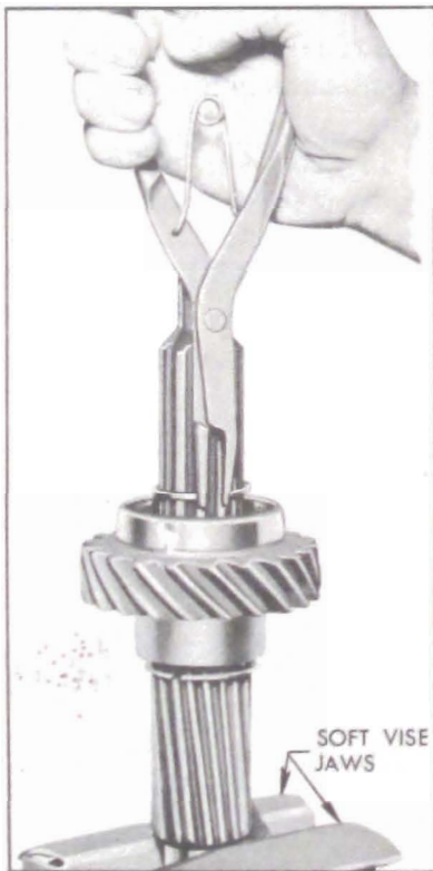
Figure 4-51—Removing Snap Ring from Main Shaft
