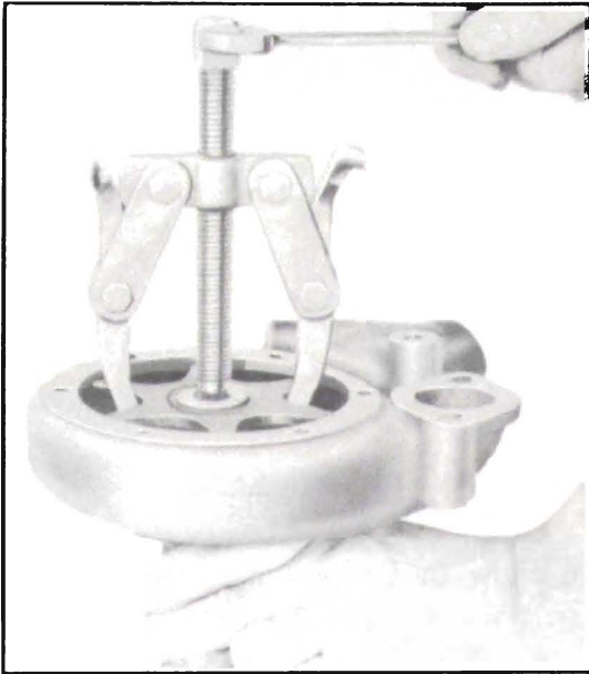
Figure 2-42—Removing Pump Impeller
