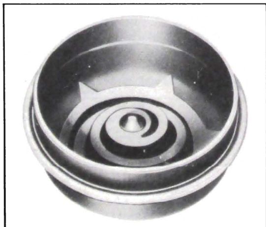
Figure 11-13—Static Collector Installed in Front Hub Grease Cap
