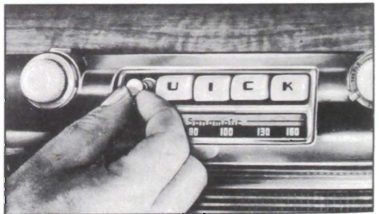
Figure 11-3—Loosening or Tightening Push Button Screw—1948 Models
