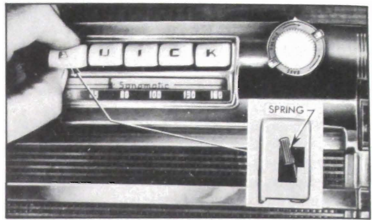
Figure 11-2—Removing Radio Push Button—1948 Models
