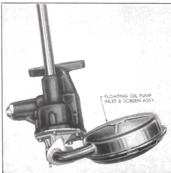
Fig. 6-39. Oil Pump Floating Screen
