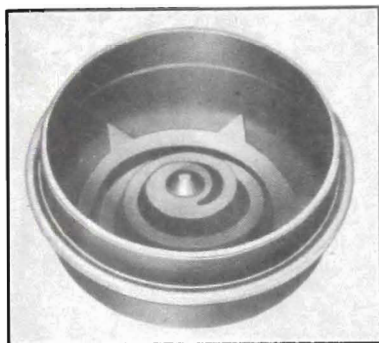
Fig. 12-114. Static Collector Installed in Front Wheel Dust Cap
