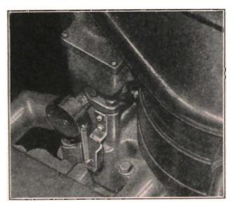
The use of the lock-out is to prevent the rear carburetor from operating on cold engines until after the automatic choke on front carburetor has reached its near open position.
