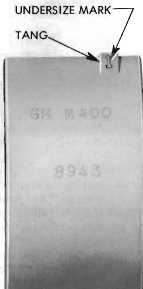
Figure 60-91 - Location of Undersize Mark on Bearing Shell
