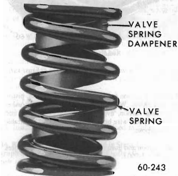
Figure 60-80 - Intake Valve Spring (350 cu.in.)
