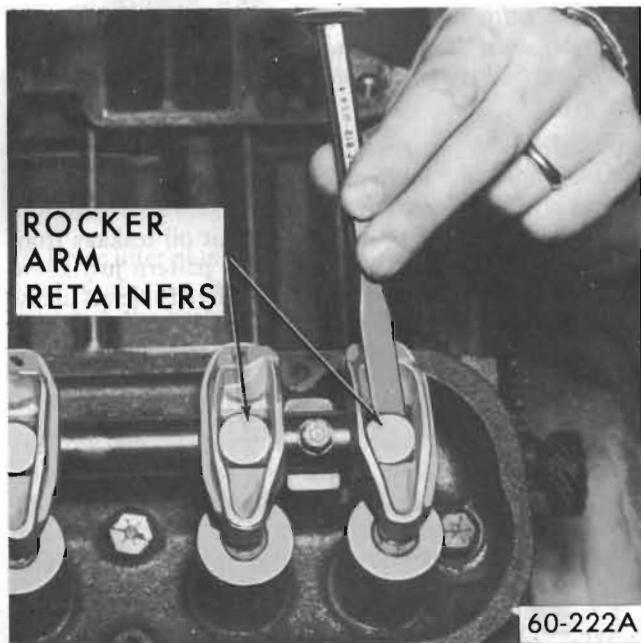
Figure 60-82 - Removing Nylon Retainer
