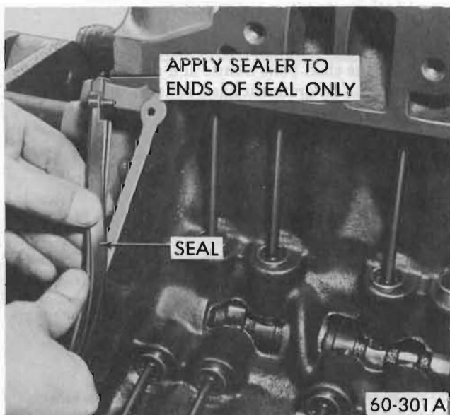
Figure 60-73 - Intake Manifold Seal Installation
