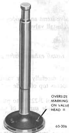
Figure 60-79 - Oversize Valve Identification
