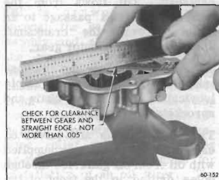
Figure 60-346—Checking Oil Pump End Clearance
