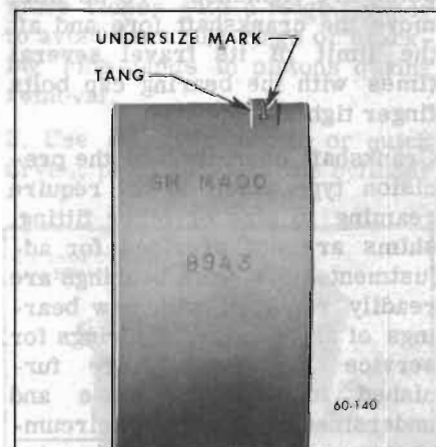
Figure 60-325—Location of Undersize Mark on Bearing Shell
