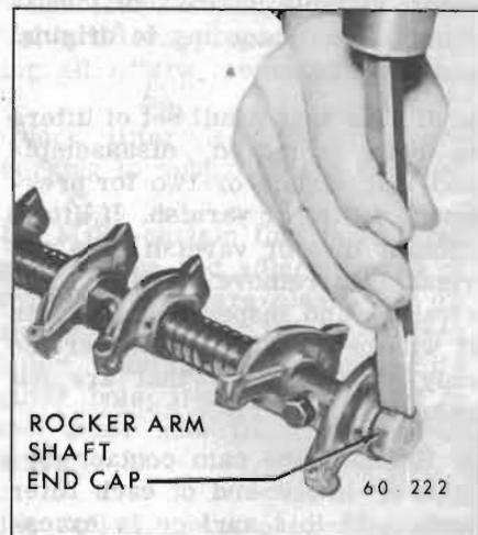
Figure 60-317—Removing Rocker Arm Shaft End Cap
