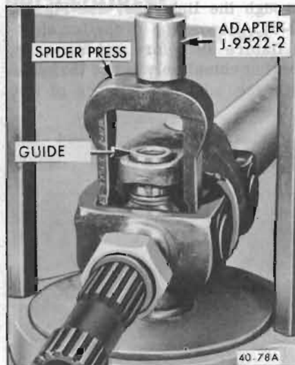
Figure 40-66—Removing Bearing with Guide and Spacer in Place
