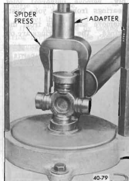
Figure 40-67—Pressing Out U-Joint Bearing
