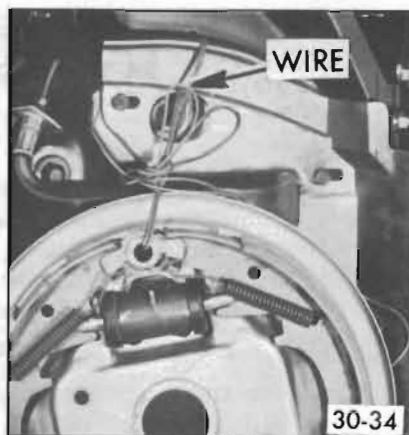
Figure 30-34—Wiring Brake Backing Plate Out of Way
