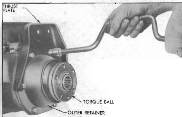
Figure 4-85—Removing Torque Ball
